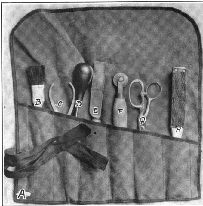
Fig. 2—A, folding case; B, brush; C, pliers; D, hook; E, skiver; F, marker; G, shears; H, roughener
